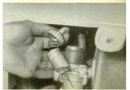
Fig. 14.Remove carburetor starter slide(choke piston)and wrap it in a clean cloth. (open ended spanner 11 mm) 15.Detach exhaust flange from engine. (socket spanner with universal joint 12 mm) 16.Disconnect the silencer from its rear attachment. (socket spanner 10 mm with ratchet. ring spanner 10 mm for counteracting on unscrewing) flange.
