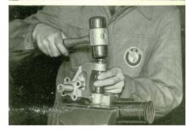
Fig. 15 39.Press out, respectively drive out the king pin bearing bushing.
