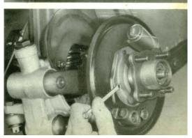
9 - Remove dust cover and oil seal assembly from backing plate only if inner ball bearing is left on wheel spindle and if oil seal or ball bearing have to be checked.
