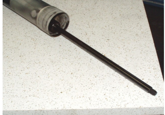
Gas spring body (with smaller washer assembly hidden) inserted into inner sleeve.
