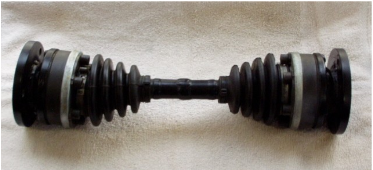
Volkswagen CV Joint Assembly with shortened shaft and the addition of new flange adapters to each end.
