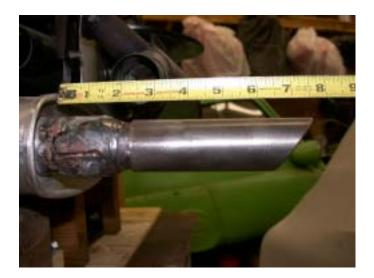
Using a 1 3/8" tail pipe (or the remaining section of the VW tail pipe) weld an extension onto the outlet of the muffler. The overall length of the outlet pipe should be approximately 8".
