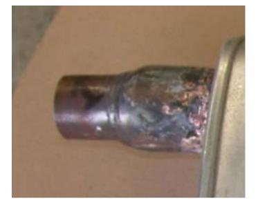
Using the section of the tail pipe marked "1", remove the mounting flange with a side grinder or chisel. Cut one or more additional slits in the larger end of the tail pipe piece similar to the factor slit. This will allow you to close the gap between the tail pipe and the muffler outlet pipe. Weld up the connection.
