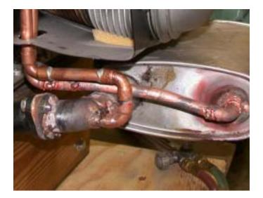
Now fabricate the 2 sets of pipes as shown in the photo to the left. The two 90 degree elbows shown in the far left should be positioned just below the opening in the cooling shroud. The joints for these pipes may be soldered instead of brazed if you so desire. The upper joints for the two elbows shown in the far left should not be soldered or brazed – they should be left as a slip fit on the two tubes coming down from the manifold.
