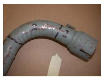
Cut the VW tail pipe at the two black lines. The "2" section will form the tight bend between the exhaust pipe on the engine and the muffler. The end closest to the "1" section will be inserted into the muffler inlet pipe.
