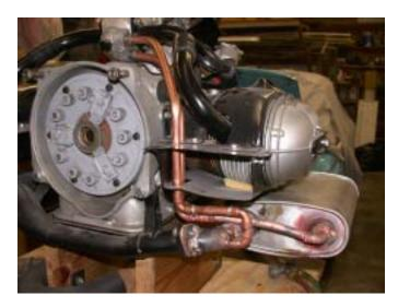
When complete you will now have a system which will provide pre-heat to the manifold. The exhaust gasses are supplied by the higher pressure located in the exhaust pipe entering into the muffler. The gasses will pass through the manifold and will exit at the lower pressure pipe located near the outlet of the muffler.
