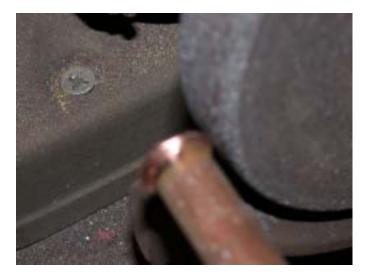
Grind the edge of the flared and flattened tube to allow it to fit freely into the housing.
