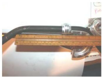
The tube is also mounted so that the center of the previous bend is 4-3/4" from the new bend. The tube should again be bent to a 50 degree angle.
