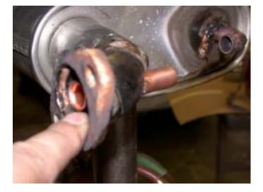
Insert the nipple into the hole drilled into the elbow from the flange end with the flared end exposed to the exhaust gasses that will be flowing in the pipe. Braze the copper tubing at the connection between the steel elbow and the copper tubing.
