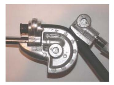
Measure in 1 - 3/4" from the flared end; this point should be at the 0 degree mark on your bender. Bend the tubing slowly in short strokes until the end is at a 50 degree angle.
