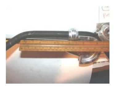
The tube is also mounted so that the center of the previous bend is 4-1/2" from the new bend. The tube should now be bent to a 50 degree angle.
