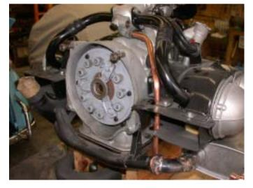
Now slide the tubing nut over the bends and install the tube in the lower rear position. Check the distance to the 90 degree fitting on the muffler pipes (not shown in this picture) and cut off the excess tubing so that it will fit into the muffler's fittings.
