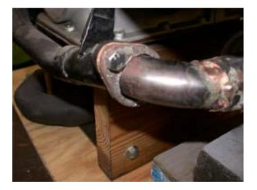
After the rear hanger has been installed, it is time to install the front flange on the inlet pipe. Using a fabricated flange or one taken from an old VW exhaust system, install the flange on the pipe and bolt it to the engine outlet pipe. Once everything is aligned, tackweld the flange to the pipe and then complete the welding on the bench.
