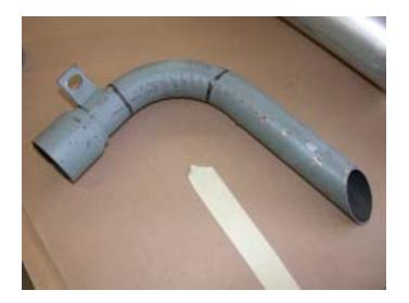
The Type III (Fastback or Squareback) VW tail pipe used in the late 60's to early 70's works well as prefabricated parts for making the tight bend and reducer pipe for the transitions pieces. If you cut the pipe in the places shown by the black lines you can use the curve piece and the reducer to lessen the work required to fit your stock muffler to your 600. Again, the VW part number for this item is 311.251.185.
