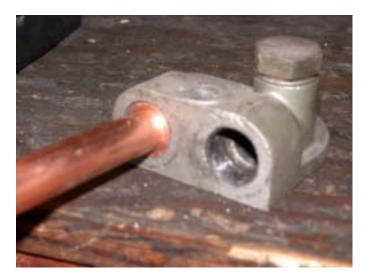
The flatten end of the tube must fit freely into the housing. Check the fit and using a grinder, remove the amount of material necessary from the end of the tube to allow for proper fit.
