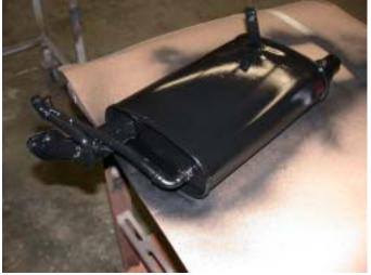
Paint the muffler with a heat resistance paint to match the original design and camouflage the fact that it is not an original!
