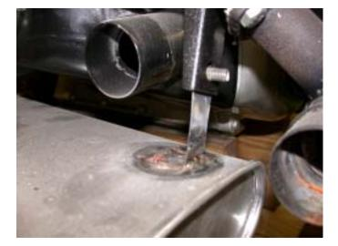
This photograph shows the hanger after being installed. Make sure that you have sufficient clearance between the muffler / tail pipe and the paper heater tube that connects from the air duct opening shown just behind the hanger to the exhaust heat exchanger. In my engine, the muffler slants slightly downwards in the rear of the engine for proper clearance.
