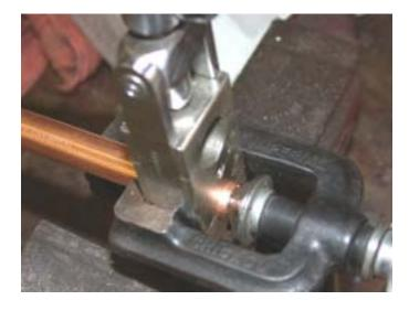
Place about 1/8" of material beyond the flaring clamp and flare the end. After the end has been flared, use a small hammer to flatten the flared end against the clamp.
