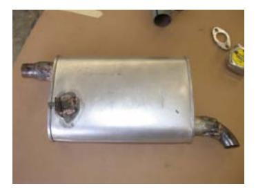
The above picture shows the muffler with inlet and outlet ports at opposite sides of the muffler. This picture was taken after the muffler had been modified with a curved inlet and a reducer installed on the outlet. Also, on the bottom left of the muffler a mounting bracket has been attached.
