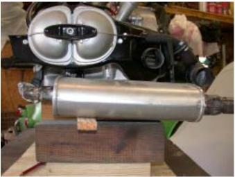
Fabricate and install a hanger for the rear of the muffler. This is done best by aligning the muffler to the engine to make the final decision on its exact location and length. In general, the bracket should be about 1" wide and a total length of approximately  $3 \frac{1}{2}$ ". One inch of the bracket should be bent at 90 degrees to provide a surface to attach the bracket to the muffler.
