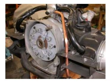
Again, slide the tubing nut over the bends and install the tube in the upper front position. Check the distance to the 90 degree fitting on the muffler pipes (not shown in this picture) and cut off the excess tubing so that it will fit into the muffler's fittings.
