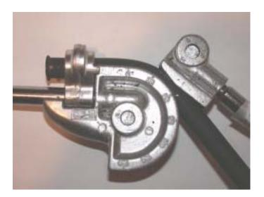
Measure in 1- 7/8" from the flared end; this point should be at the 0 degree mark on your bender. Bend the tubing slowly in short strokes until the end is at a 50 degree angle from the centerline of the flared end.
