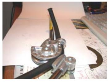
The next bend is made at an 80 degree angle to the first. Note the position of the flared end in the bender. It is mounted so that it is angled at 10 degree from vertical.
