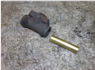
Once the cylinder has been drilled, cut a length of brass tubing slightly longer than the length of the cylinder. I used a dermal tool for this to prevent any deformation of the tubing.
