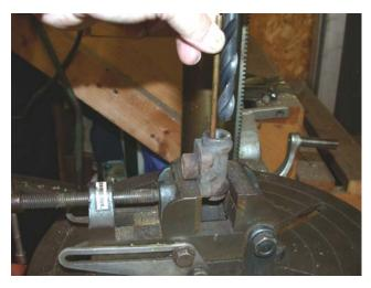
Use some type of straight edge and make sure the cylinder is true with the drill. Check the squareness in both the "X" and "Y" axis. After you are certain all is true bolt the vice down to the drill press (if possible). This last part is not completely necessary, but it does afford you some safety in the event the drill catches in the cylinder.
