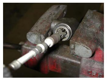
On the larger front cylinders, use a cylinder hone to clean up any burrs on the cylinder wall from the drills. Also make certain you clean the edges where use used the dermal tool to dress down the ends of the brass tubing.
