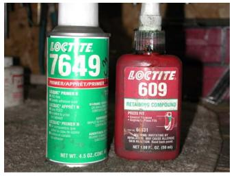
Using Loctite cleaner–primer, prime both the inside of the cylinder and the exterior of the brass tube. Allow the primer to dry as instructed on the container.
