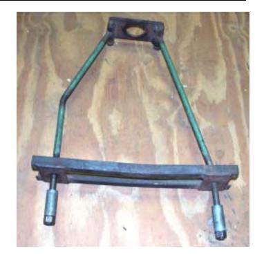
The top plate is 2-3/4" wide x 5" long x  $\frac{1}{4}$ " thick. It has a hole in the middle 1-3/4" in diameter. This hole secures it to the spring housing and keeps it from slipping off when being used.
