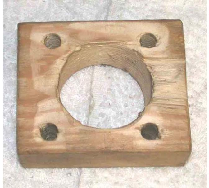
When using the tool, (1) steel plate is secured at one end, (1) wooden block is secured near the top of the painted end of the spring housing. The other wooden block and steel plate slide towards the stationary block / plate as the nuts on the threaded rod are tighten. The wooden block that is not secured must be moved by hand as the spring is compressed.
