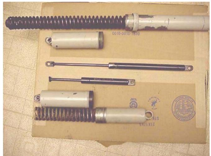
If you are having trouble with your door staying open, you might consider installing one of these gas struts. On the Isetta 300 you can purchase one made to fit into the spring housing directly from Werner Schwark at
